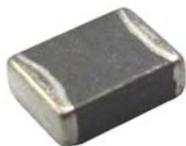
The MPL Series is a miniature type of multilayer power inductor constructed using low-loss ferrite material to support high-speed switching frequencies. The compact size and high efficiency is ideal for DC-DC converter applications in space-limited boards.
